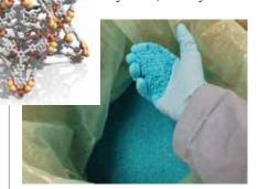
▲ NuMat designs and produces MOFs porous structures comprised of metal ions (orange) linked together with organic molecules (gray, red) — for gas storage and separation. The company can produce a granulated MOF product (blue powder) using a scalable pre-pilot process with a capacity of 20 lb/day.
