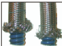
Hastelloy (left) and stainless steel hoses appear identical.
