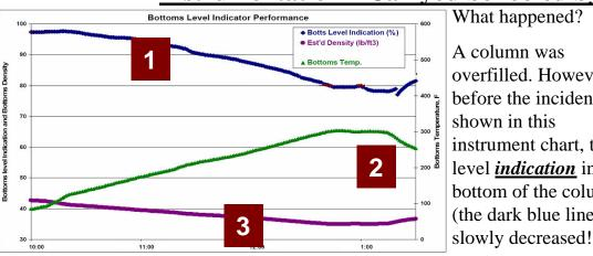
A column was overfilled. However, before the incident, as shown in this instrument chart, the level *indication* in the bottom of the column (the dark blue line - 1)
