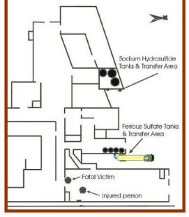
had ever received on his shift. He directed the truck driver to the unloading station for ferrous sulfate, where the truck is shown in the diagram. The shift supervisor did not verify the identity of the chemical in the truck, although the shipping papers did properly identify the contents as sodium hydrosulfide. The supervisor signed the shipping papers without reading them and left the area. No plant employees remained in the unloading area.
