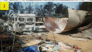
In July 1948 a tank car filled with dimethyl ether (DME) arrived at a factory in Ludwigshafen, Germany. It stood in sunlight for about 10 hours when it is believed that a weld seam failed. About 200 people were killed, nearly all by the explosion of the flammable DME vapor cloud created by the leak. Nearly 4000 people were injured, the majority by exposure to toxic substances escaping from installations damaged by the blast (Picture 1).
