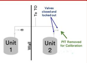
Units 1 and 2 share a common line to the thermal oxidizer (TO). Calibration was due on several instruments on unit 2. A hand valve was closed and locked out, and a pressure transmitter (PIT) was removed for calibration.
