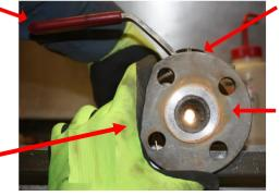
Valve handle failed and allowed handle to turn without closing the valve
