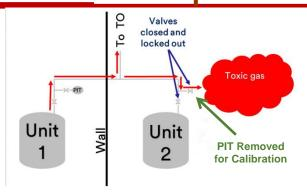
A day or two after unit 2 was locked out, unit 1 began venting toxic gas through the shared line to the thermal oxidizer. The material venting from unit 1 flowed through the vent line toward unit 2. However, the material exited through the valve where the pressure transmitter had been removed.
