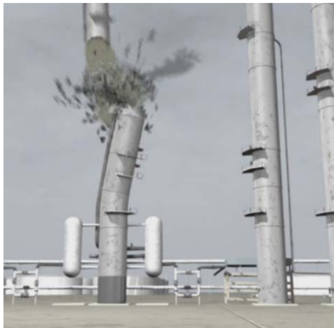
Screen capture of the explosion in the US CSB animation video of the incident (CSB REPORT NO. 2003-01-I-MS)
