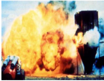
Figure 2: Vented dust continues to burn outside of the vessel
