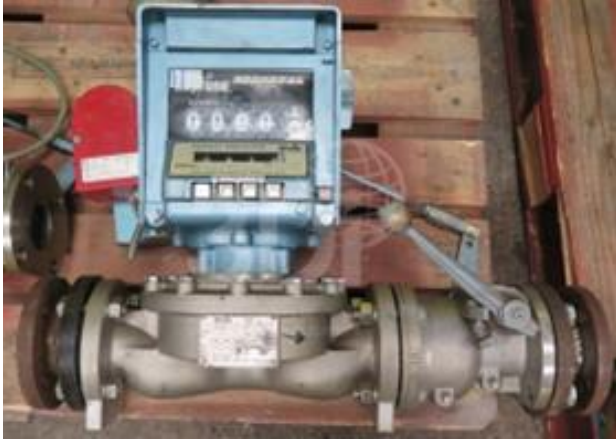
Figure 1. Flowmeter ready for calibration
