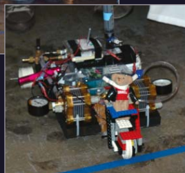
Evidence of perfection: Cornell Univ.'s "Bender" — a hydrogen fuel cell car with an iodine clock stopping mechanism — won the Chem-E-Car Competition, stopping exactly on the target line of 60 ft.
