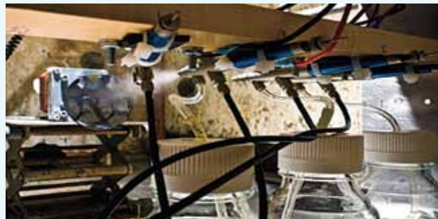
▲ In this automated LbL setup, nozzles spray separate streams of both positively and negatively charged species, as well as a rinse stream used between each adsorption step. Image courtesy of MIT Press.
