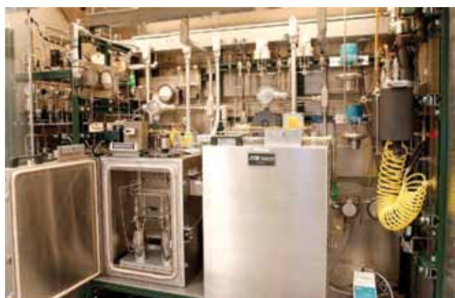
▲ Figure 7. These two ovens are being used as heated enclosures.
