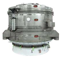
The K100-2(IRC)-SS round vibratory screener separates oversized particles from bulk materials at rates of up to 150 tons/hr. The screener includes a large, 75-ft<sup>2</sup> screening area and is totally enclosed for dust-tight operation. Above the conventional screen is a slightly smaller, high-capacity Kascade Internal Recycle screening deck comprised of two screens of the same mesh operating in series. This
