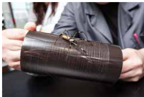
▲ Researchers have cloned the protein used by the orb weaver spider to make a variety of materials, including the synthetic fibers shown here. They have spun silk fibers more than 1,000 m long.
