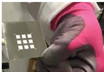
▲ Cold sintering creates composite materials with lower energy costs, such as \text{Li}_2\text{MoO}_4 capacitor structures on nickel foil, which is sintered at 100 MPa for 15 min at 120°C.
