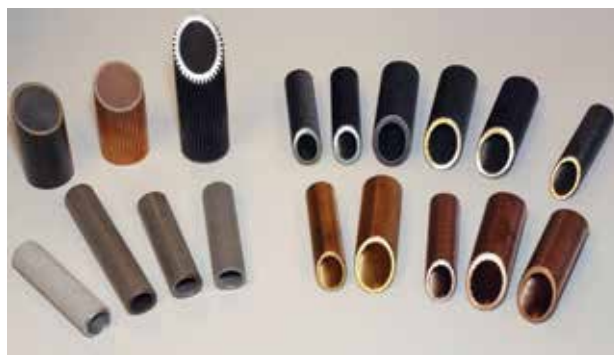
▲ Figure 7. Enhancements to the design and texturing of reboiler and condenser tubes (HighFlux or HighCond) significantly improve heat-transfer rates by reducing the resistance on the convective side and improving the management of surface temperatures. Photo courtesy of UOP.
