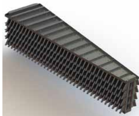
◀ Figure 4. Schoepentoeter-Plus is an advanced centrifugal device for deentrainment and vapor distribution commonly used for two-phase feeds into distillation columns. Figure courtesy of Sulzer Chemtech.
