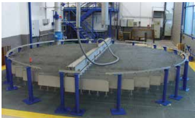
▲ Figure 5. This modern liquid distributor (shown here on a stand for testing) increases column efficiency. Photo courtesy of Montz.
