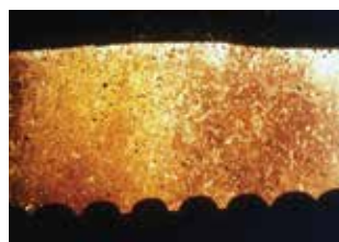
◀ Figure 8. Sawdust and wood chips are fed to a furnace at a paper mill. The view through the sightglass into the spreader-stoker indicates the furnace temperature. The yellow and white areas are hotter, while the darker spots are cooler wood particles.
