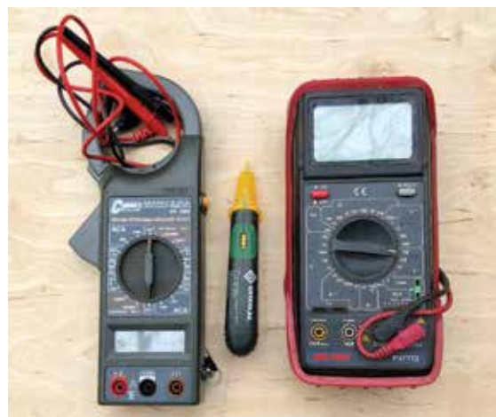
▲ Figure 6. In the field, it is often useful to take electrical property measurements using instruments such as an amprobe multimeter (left), noncontact hot-wire tester (center), and multimeter that accepts a Type K thermocouple input (right).
