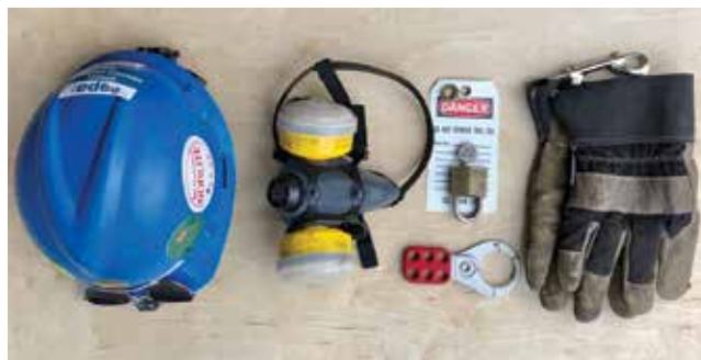
▲ Figure 2. Important safety gear that any troubleshooter should have on hand include (from left to right): hardhat, dual-cylinder air-purifying respirator, lockout/tagout gear, and leather-faced insulated gloves.
