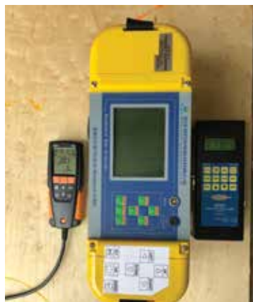
◀ Figure 9. A troubleshooter may use various handheld instruments such as these to test stack emissions.
