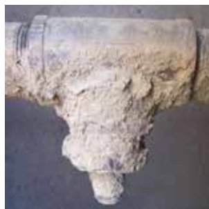
◀ Figure 10. Spray nozzles often foul and plug, as has occurred here due to lime fouling.
