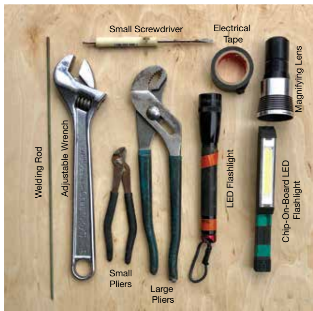
▲ Figure 4. These hand tools belong in any troubleshooter's gear case.
