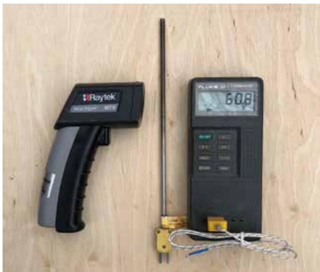
▲ Figure 7. These common instruments can be used to measure temperature in the field (from left to right): infrared (IR) noncontact thermometer, Type K thermocouple (TC), and dual-channel field TC readout.
