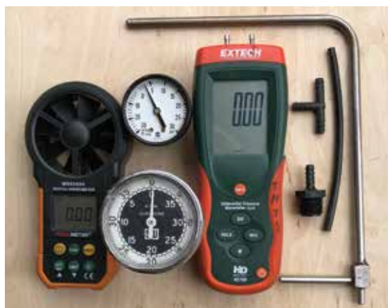
▲ Figure 5. Instruments for measuring flow and pressure include (from left to right): velometer, compound gauge (top), mechanical tachometer (bottom), digital manometer, adapter, plastic tee and hose, and stainless steel pitot tube.
