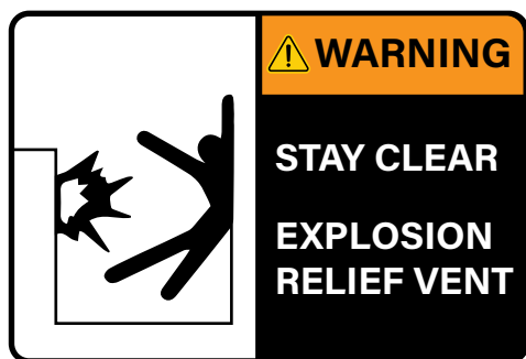
▲ Figure 2. Ensure that explosion relief panels are properly labeled.
