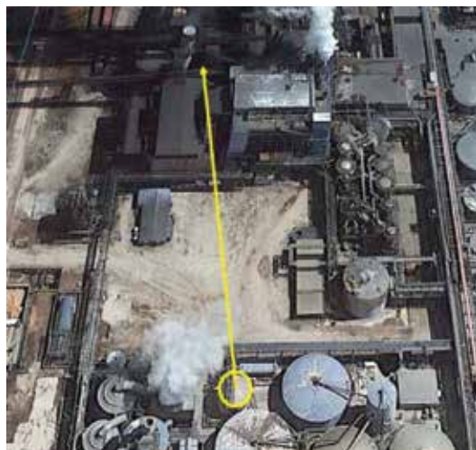
▲ A foul condensate tank exploded at a mill and traveled 375 ft (yellow line) before landing on process equipment. Image courtesy of the U.S. Chemical Safety and Hazard Investigation Board.
