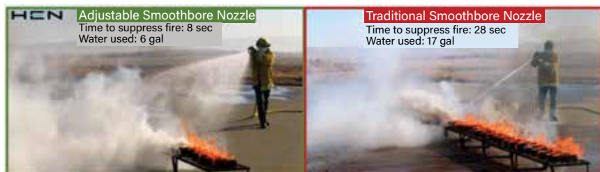
▲ The blade pattern of the HEN nozzle was able to suppress a fire in eight seconds using six gallons of water (left). This suppression rate was three times faster than the traditional smoothbore nozzle (right).
