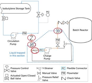
▲ An incident occurred in a process with an inaccurate piping and instrumentation diagram (P&ID). Image adapted from the U.S. Chemical Safety and Hazard Investigation Board (CSB) Report No. 2019-02-I-TX.
