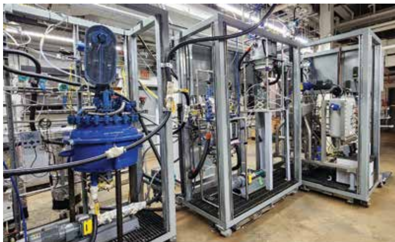
▲ Figure 3. The buildout of the demonstration skid units is shown with the reaction skid, crystallization skid, and filter/drying skid lined up from left to right.
