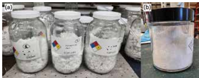
▲ Figure 4. (a) Wet cake pharmaceutical raw material is produced directly from the skid process. (b) The recrystallized and fully dried sample contains <1 ppm measurable impurity.
