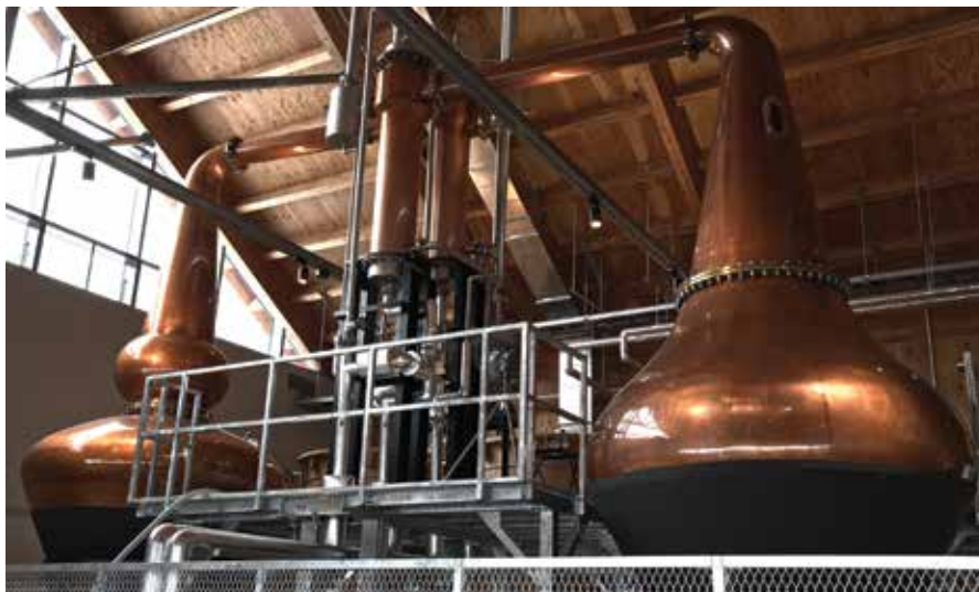
▲ Figure 3. Copper stills at a whiskey distiller refine and concentrate the fermented liquid.
