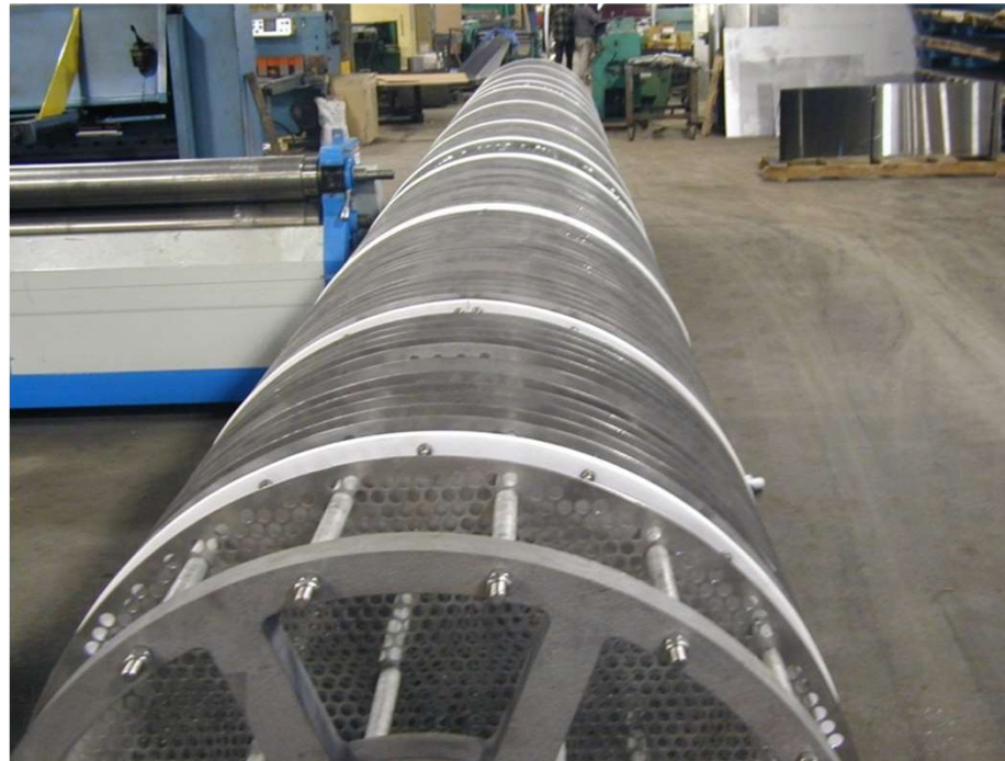
Internals for a 3 foot (1 meter) diameter KARR® Column
