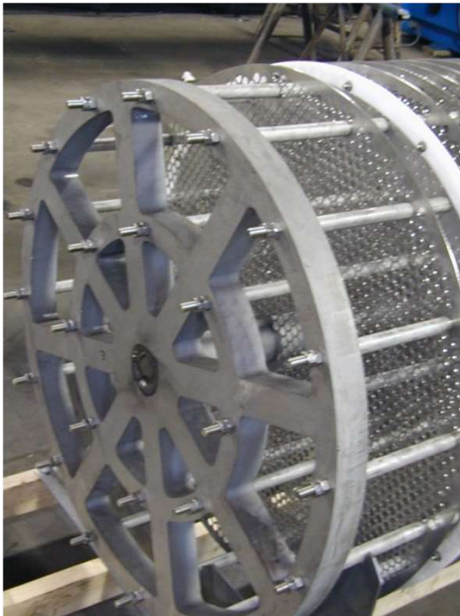
Internals for a 3 foot (1 meter) diameter KARR® Column
