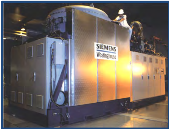
Siemens/Westinghouse 220 kW Pressurized SOFC/GAS Turbine Hybrid System
