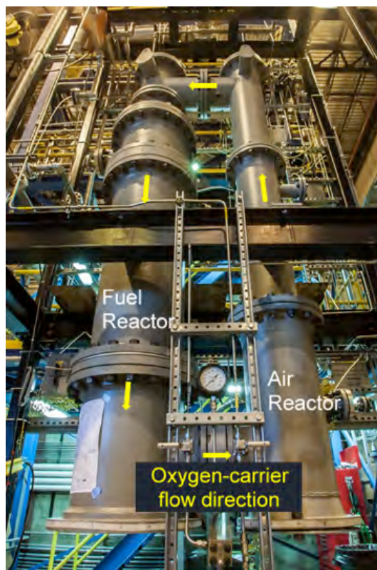
NETL's 50 kW chemical looping reactor. In the fuel reactor (left), a fuel such as methane reacts with an oxygen-carrier material. The reduced oxygen carrier is sent to the air reactor (right) where it is regenerated to its oxidized state. Then the oxygen carrier is returned to the fuel reactor. Courtesy: NETL
