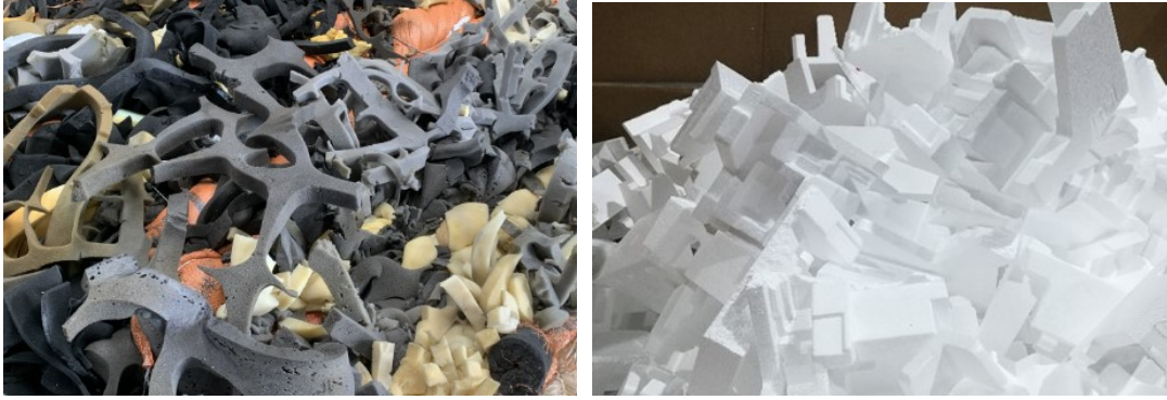
Figure 7: Typical shredded polyurethane and polystyrene foam
