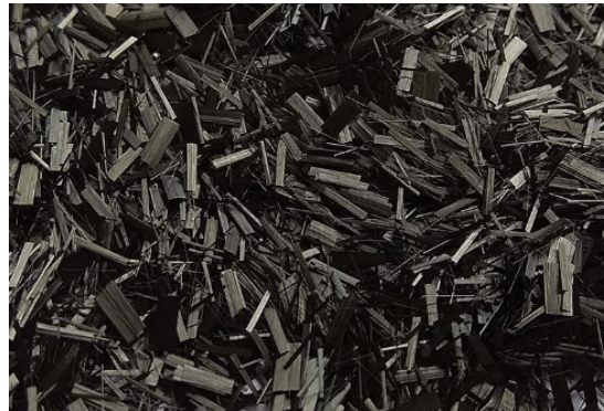
Figure 8: Typical regrind with carbon and glass fiber reinforcement
