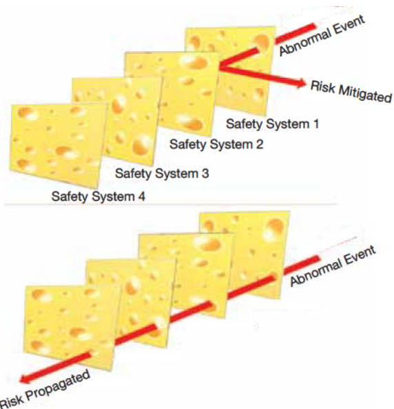
▲ Figure 1. The Swiss cheese model illustrates that when the weaknesses in layers of protection align, an accident can occur.
