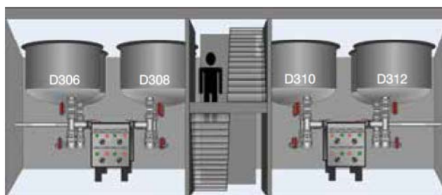
▲ Figure 7. Reactors D306 and D310 occupied the same place in their respective, identical tank rooms. At the bottom of the stairway, the operator became confused and went into the wrong room, where he emptied the wrong reactor. Source: (7).
