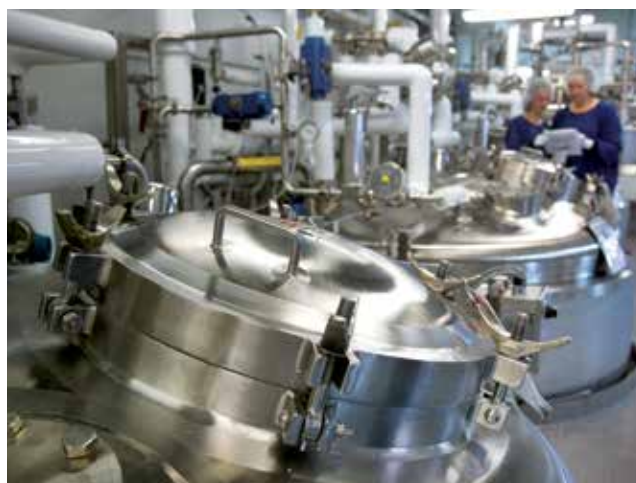
▲ Figure 4. A typical biomanufacturing plant can take over two years to design and construct, and must be thoroughly cleaned in between every product run. The manufacturing plant shown here produces therapeutic proteins in bioreactors that measure 25 m 3 . Image courtesy of Bristol-Myers Squibb.
