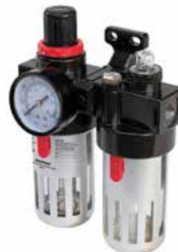
► Figure 7. The plastic bowls on the bottom of filter/regulator/lubricators (FRLs) are notorious for leaks. Establishing a formal air leak search, tag, and repair program can help document and remedy FRL leaks.
