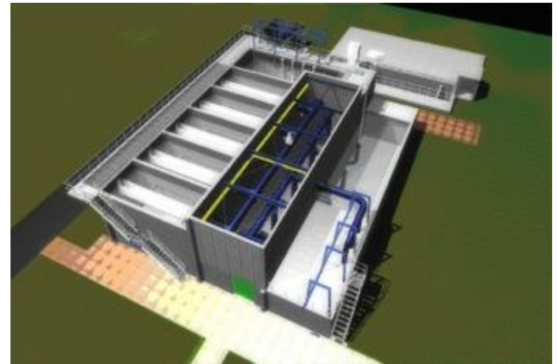
1-Step filter wwtp Horstermeer
