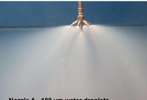
Nozzle A - 100 µm water droplets Nozzle B - 200 µm water droplets - •K
