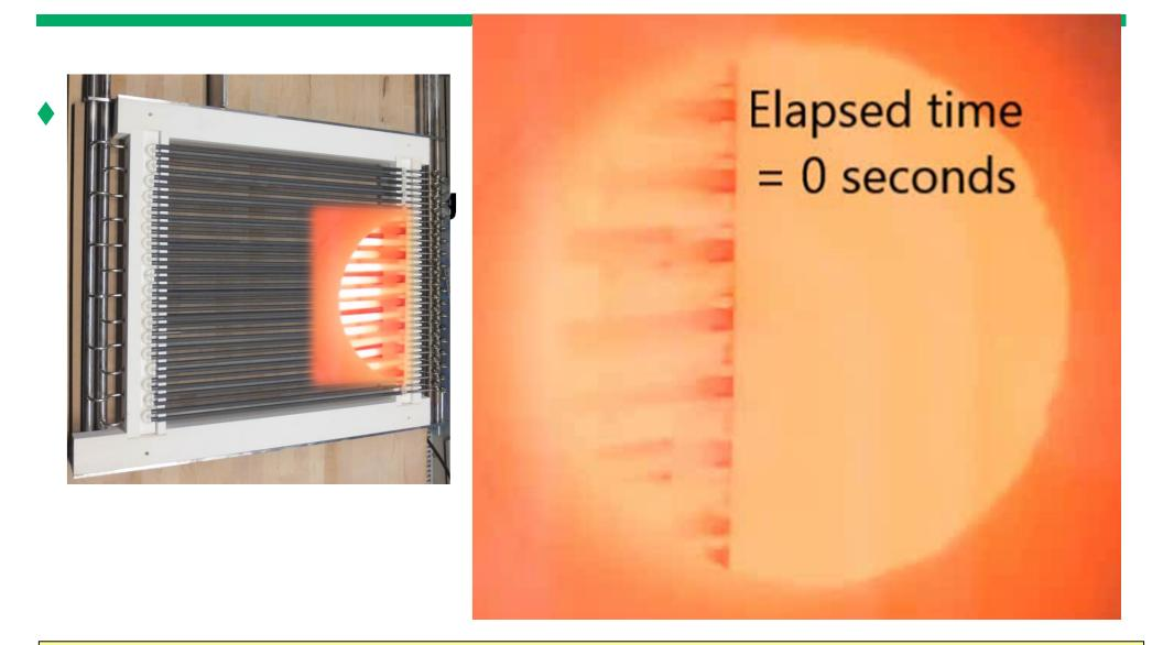
Syngas module robust to thermal cycles, trips, and transients
