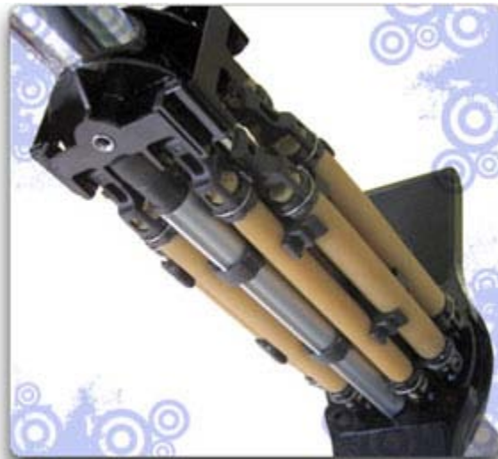
Figure 12: The elastic mechanism within a Flybar pogo stick.
