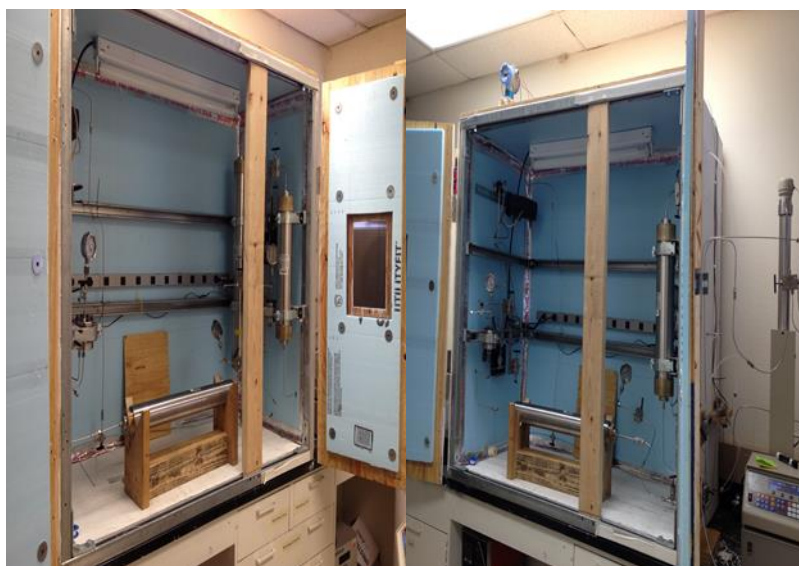
Fig. 4 The schematic diagram and pictures of the core flooding apparatus.
