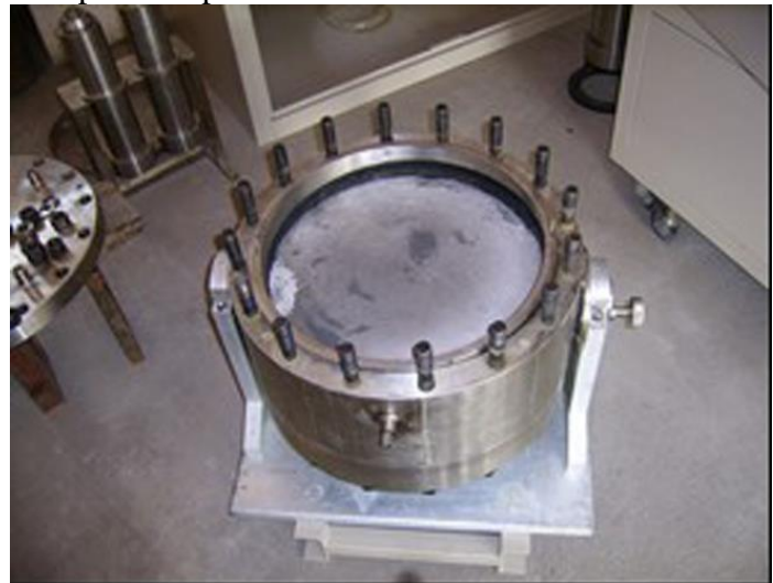
Fig.2 Coreholder of 3D physical model
