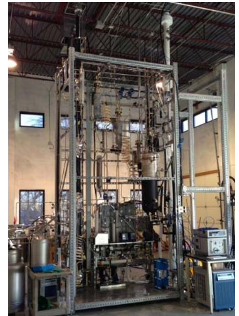
ION's 0.01 MWe CO 2 capture lab pilot unit
