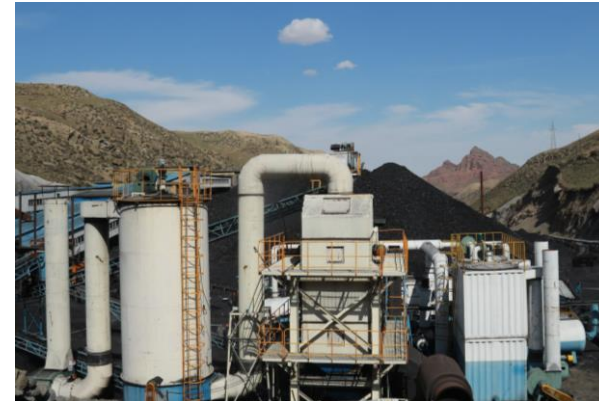
Fig. 3.11. Modular Air Dense Medium Fluidized Bed Industrial Separator
