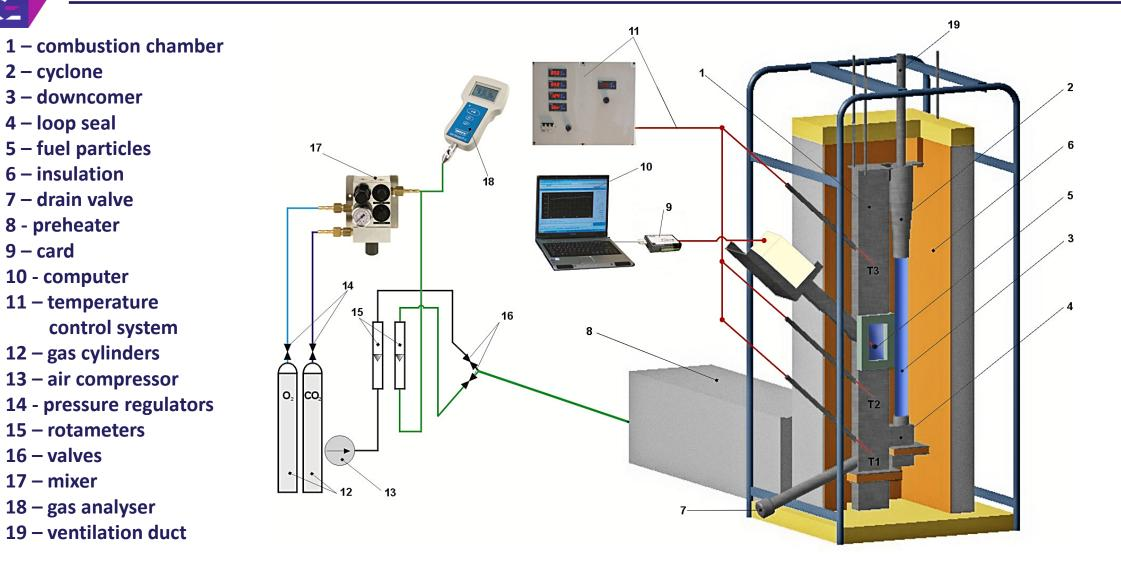
T1–T3 – S-type thermocouples
